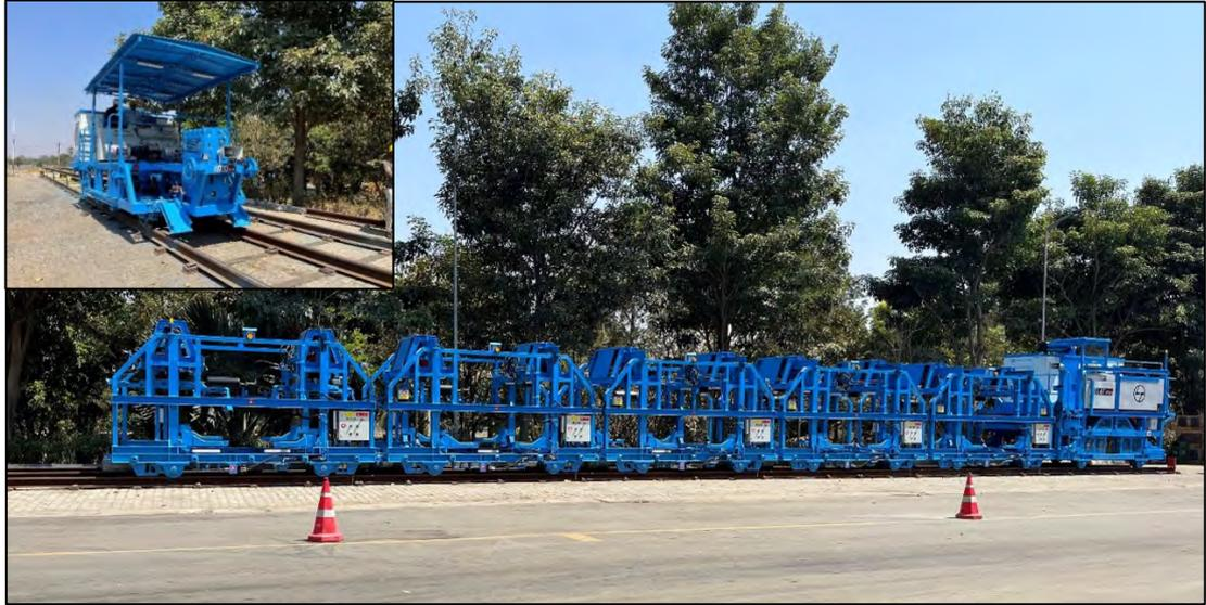
*Track Works (package T2) -- Track Slab Laying Car and Rail Laying Car (In inset), Gujarat*
