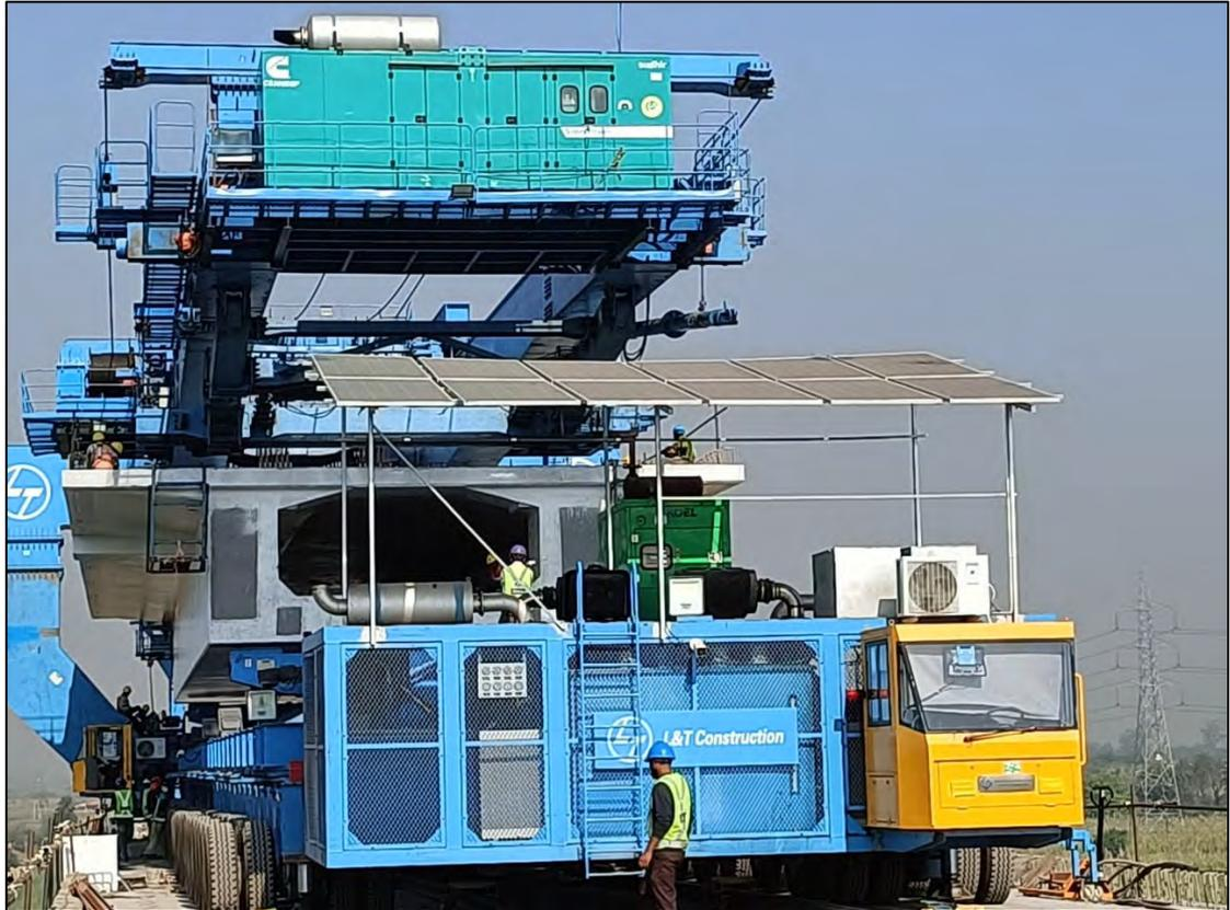
*Solar Panel Provided on Girder Transporter To Power A/C of Operators Cabin*
