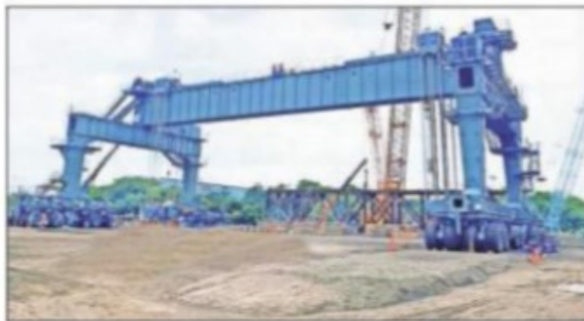
The straddle carrier is a tyre mounted self-propelled gantry crane with a capacity of 1,100 MT; (Below) The girder transporter is designed to transport the full span precast girders. Courtesy: NHSRCL
