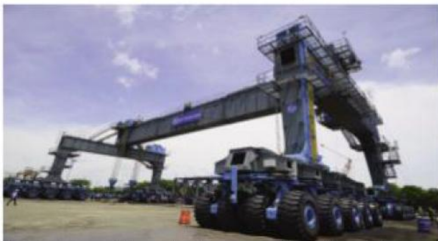
The equipment will expedite the process of launching girders
