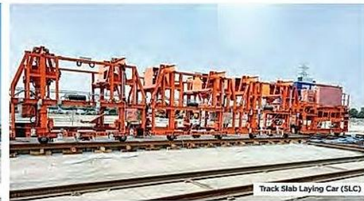
Track Slab Laying Car (SLC)
